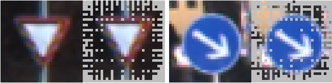
Fig. 4: Minimal sufficient feature set visualizations for GTSRB inputs. Pixels not included in the explanation are shown in gray.
